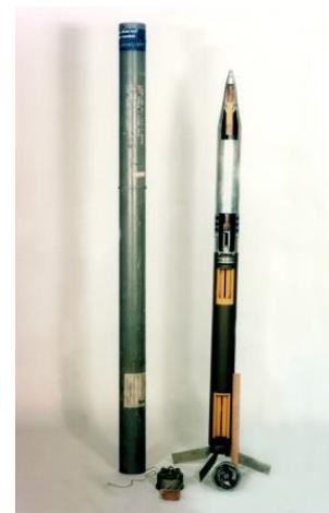
M55 rocket (right) and shipping and firing tube (left).
