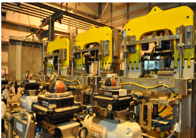
The munitions washout system (MWS) will rinse agent out of the agent cavity of nerve agent projectiles
