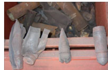
Munitions scrap metals similar to this resulting from SDC treatment, will be released for recycling at an appropriate facility.
